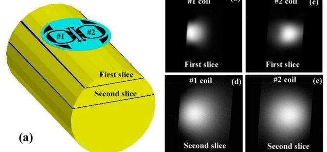
Fig. 2. (a) Configuration of the array and phantom for the coil decoupling test is shown; (b) and (c) first slice 4.7 Tesla images of the number one and number two coils, respectively; (d) and (e) second slice images of the number one and number two coils, respectively. Mutual decoupling of the both coils can be clearly seen. Note that the #1 coil was placed toward the left side of the phantom.
