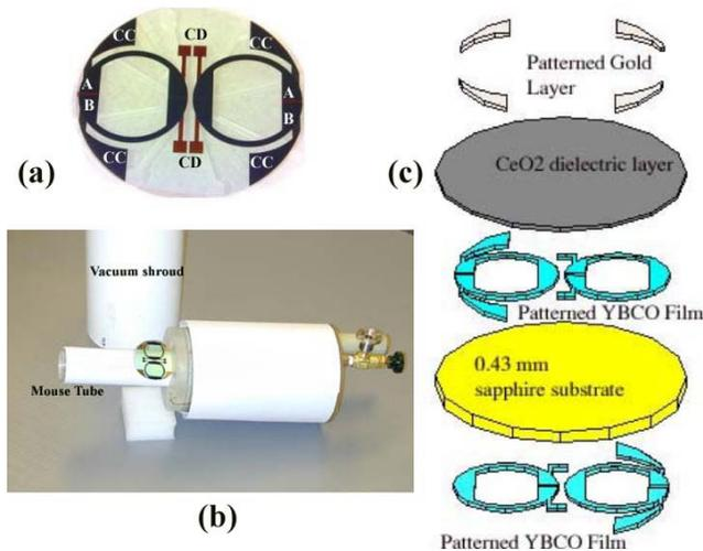
Fig. 1. (a) A picture of the upper side of an array, CC and CD denote de-coupling and coupling capacitors, respectively. A and B shows two sides of the upper quasi ring gap; (b) A picture of a part of the cryostat. The array attached to the sapphire cold-head is shown next to the mouse tube; (c) an example of the multi-layered design is shown.
