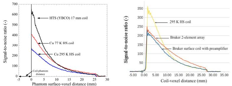
**Figure 2.** Comparison of the SNR of Cu and HTS 300 MHz coils vs. voxel distance from the phantom surface. Both copper and HTS were cooled to liquid nitrogen temperatures. Note that for reference purposes the SNR data for Bruker surface coil and array are also included in the plot (b). It provides performance comparison of the homemade.
